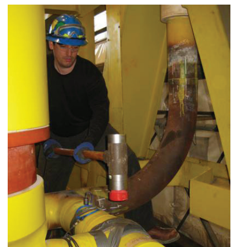
Figure 2: Impact testing of a large valve system using a modal sledge hammer.
