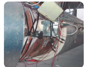
Acoustic emission probe for cracking detection.
