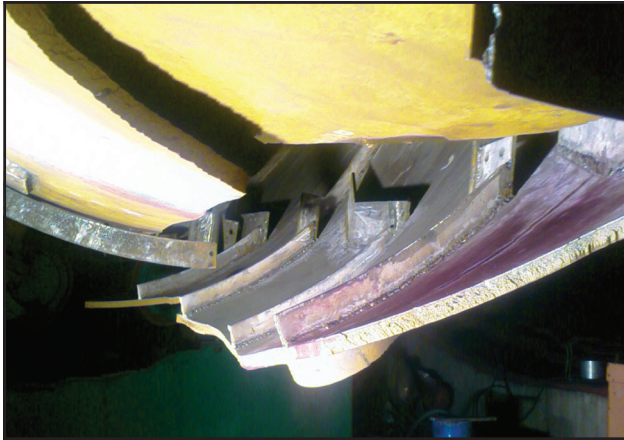
Figure 3: Brittle Fracture during pressure testing
