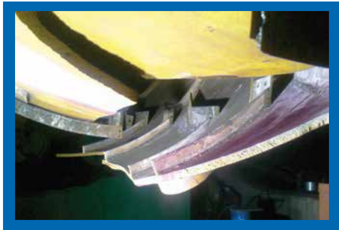
Figure 3: Brittle Fracture during pressure testing
