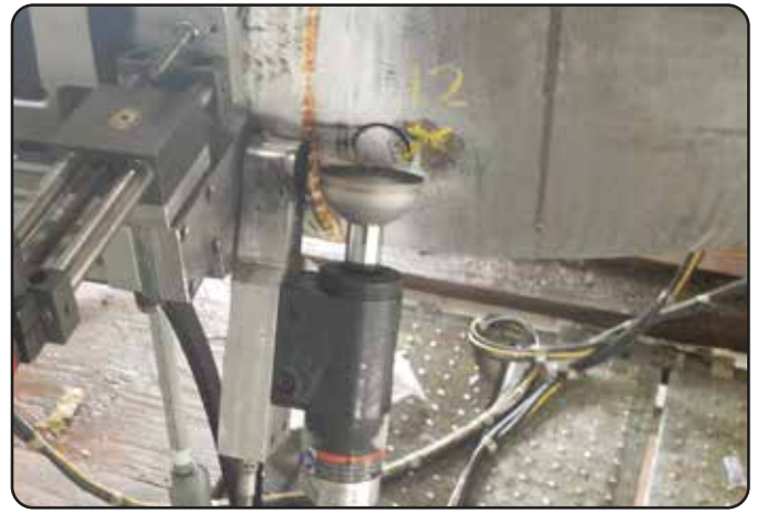
Cutting a small scoop from a high temperature pipe
