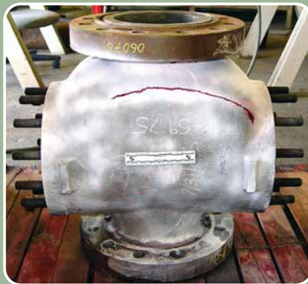
A cast 8-inch sliding stem valve body showing a through wall crack after it was tested using dye penetrant.
