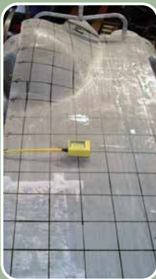
A 6-inch grid on the surface of a vessel explosion bulged aluminum plate fin heat exchanger. The grid was used to support a finite element analysis model.
