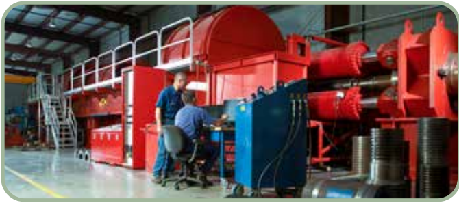
Six Million Pound Tension / Compression Test Frame
