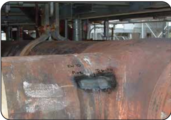
Replication site across a weld joining a large diameter tee and pipe
