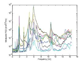
The forcing function spectrum can be estimated from the measured acceleration data and FE model. The forcing function is then applied to the jumper FE model. Resulting FE acceleration spectra are compared to the measured acceleration spectra. The left figure shows the measured acceleration spectra from nine sensors. The right figure shows the FE accelerations. This calibrated analysis results in accurate stresses and fatigue damage estimates.
