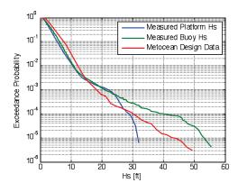
Continuous metocean and **FPS** response monitoring allows for assessment of the design environment and response. The left figure compares measured significant wave heights exceedance probability (from 5 years of FPS data, 14 years of buoy data) to metocean design data. The right figure (normalized) measured shows tendon tension standard deviation probability, exceedance along with tensions resulting from the design scatter diagram.
