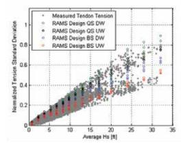
Continuous monitoring also enables investigation of FPS performance. The left figure shows the relationship of normalized tendon tension standard deviation to significant wave height over a 5 year period along with RAMS¹ predictions from the design scatter diagram.
