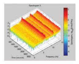
Measured jumper accelerations are examined first to determine the nature of random vibration. The left figure shows an acceleration spectrogram. The vibration is observed to be stationary over the measurement period. The right figure illustrates a normal score plot. Since the acceleration distribution falls on a straight line, the vibration is concluded to be Gaussian.
