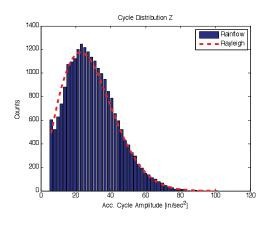
Peaks or rainflow cycles from stationary random vibration data follow a Rayliegh distribution if the vibration is also narrow-banded. The left figure compares the histogram from measured jumper vibration data to the theoretical Rayleigh curve.
