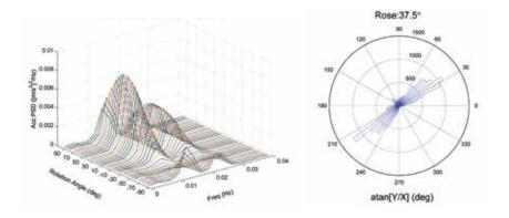
Various characteristics of riser vibrations have specific signatures in various statistics. By cross-confirming each vibration characteristic with multiple statistics, we obtain definitive conclusions on the riser behavior. Consequently, we can use the correct model to estimate extreme stresses and fatigue damage of the riser.
